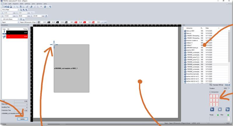
The screenshot shows the Job Control software interface. On the left, there's a 'Material Settings (of Plate)' panel. In the center, a 'Plate Laser Bed' is shown with 'Laser Position Crosshairs'. On the right, there's a 'Job Queue' list of printed files and a 'Preview' area. Arrows point from text labels to these specific parts of the interface.
